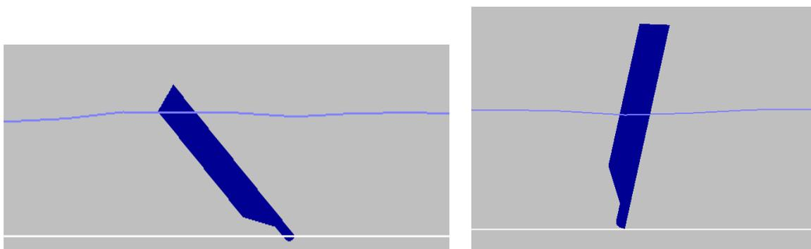
*Mean inclination of the Mose gate –  $T_p=8.0\text{s}$
