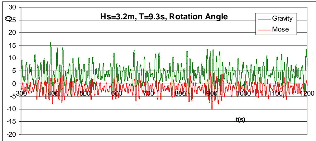
Mean inclinations are obtained :  $2^\circ$  down-lift for the MoSE gate and  $4^\circ$  up-lift for the Gravity gate. Down-lift reduces the free-board of the gate barrier, up-lift increase the free-board. Dynamic components are quite similar for the two gates with a maximum amplitude of  $10^\circ$ .
