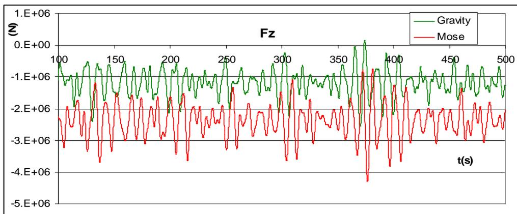
Even if rotation amplitude of the Gravity gate is larger than the amplitude of the MoSE gate, vertical force is smaller, mainly the mean wave drift force.
