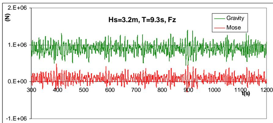
Both mean component and dynamic component are quite different compared to the linear calculations. Dynamic component is drastically reduced.
